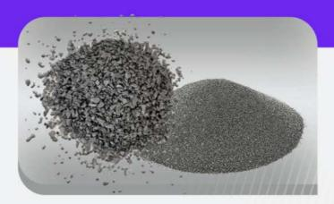
Zirconium inoculant is widely used in castings as a ladle additive or during flow, and causes uniform solidification and morphology improvement.
