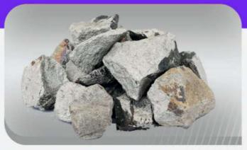
NiMg is used as modifiers in the casting of cast iron of various grades. NiMg added into the base metal during its melting.
